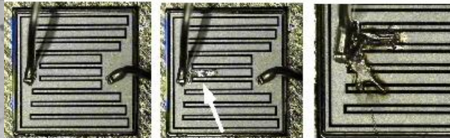
Thermal failure of the power transistor
