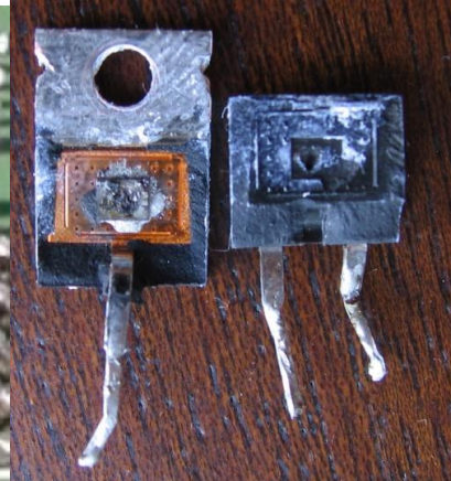
Silicon starting to melt from overload
